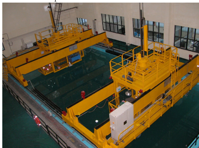
Figure 1: Acoustic test tank with transducer positioning system (ATPS).
