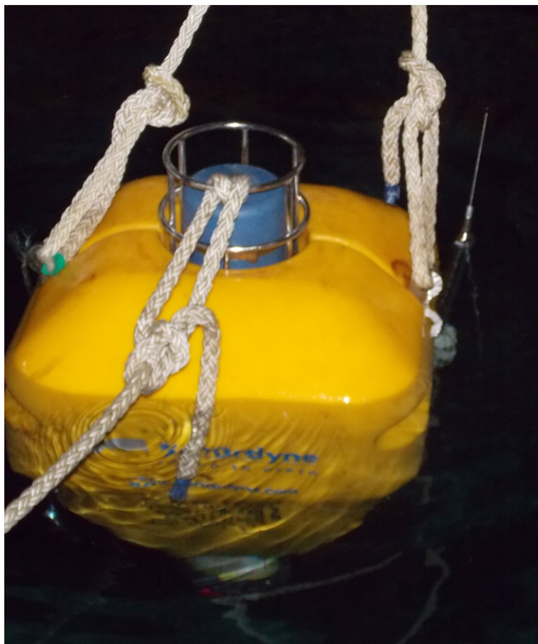
Figure 4: Tsunami Bottom pressure recorder and Ambient noise measurement system being tested at ATF.
