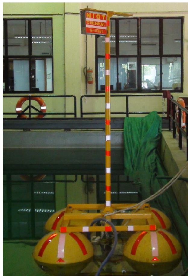
Figure 4: Tsunami Bottom pressure recorder and Ambient noise measurement system being tested at ATF.
